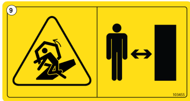
Fig. 12 Decal - Rotating parts warning, keep your distance.
