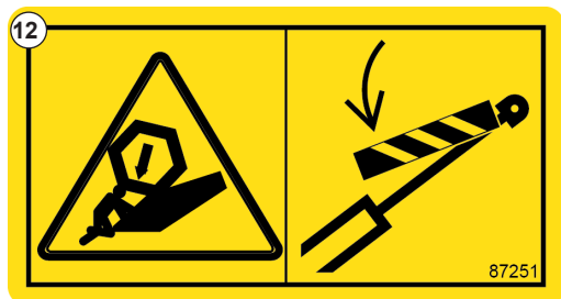
Fig. 15 Decal - Use reel arm lock before servicing
