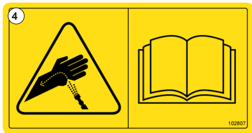
Fig. 7 Decal - High pressure fluid warning - Read manual for more details
