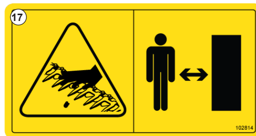
Fig. 19 Decal - Warning sharp sections
