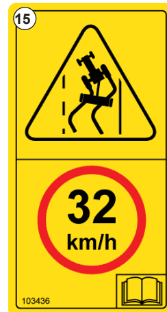
Fig. 16 Decal - Maximum transport speed
