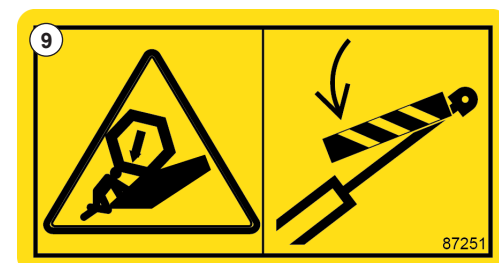
Decal. 9 - Engage reel cylinder locks before servicing - #70051
