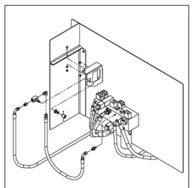
Illustration A - Page 42: Needle Valve and Hydraulid **Control Block**
