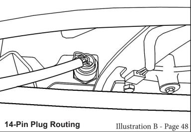
4. Insert the plug into the receptacle provided as shown to the right. First align the widest tab in the plug with the wide slot in the receptacle. Once it is fully seated, turn the locking collar to secure the plug.
