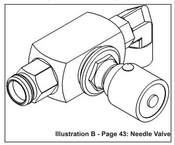
Units with serial numbers up to and including 320000 will use the needle valve assembly shown here. Use components 2, 3, 5 or 1, 7, 4 depending on the year of the Power Unit.
