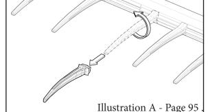
3. Reverse the above procedure to install the new reel finger.
