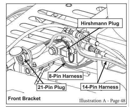
3. Feed the 14 pin plug under the front of the right side of the cab.
