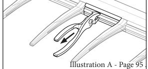
2. Twist the reel finger counter-clockwise and pull to remove it from the channel.
