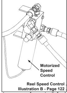
The reel circuit flow control is located on the side of the strut on the right-hand end of the table (see Illustration "B").
