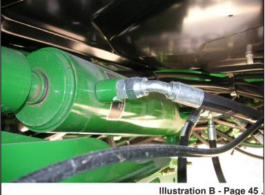
8. Install an 8MB-10MF 90° on the hydraulic cylinder port that you had removed hose "A" from in the previous step. Connect the supplied hose "B" to the fitting.
