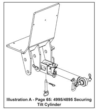
14. For all A400 and R450 tables, re-install Pin 1 (as shown to the right) to secure the cylinder mounting bracket in place.
