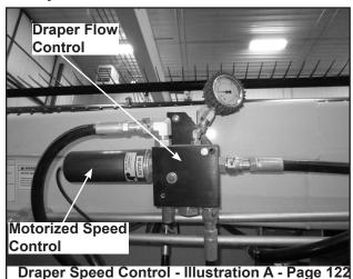
The draper circuit flow control is located on the upper tube on the left-hand end of the table (see Illustration "A").
