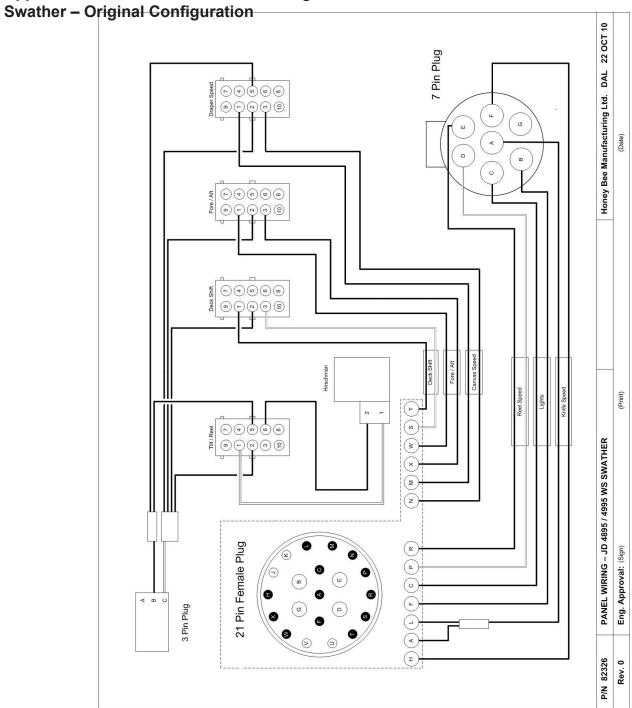
Applicable to all JD 4995 units with serial numbers before E04995X330675 and all JD 4895 units with serial numbers before E04895X330107.
