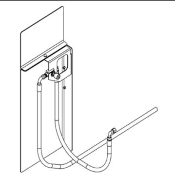
Illustration B - Page 41: Needle Valve Bracket - Installed
