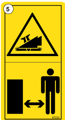
Fig. 8 - Crush warning keep safe distance - #87233
