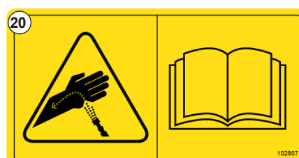
Fig. 23 - Do not pressure wash this area - #89333
