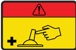
Fig. 138 - Warning! Add air!
