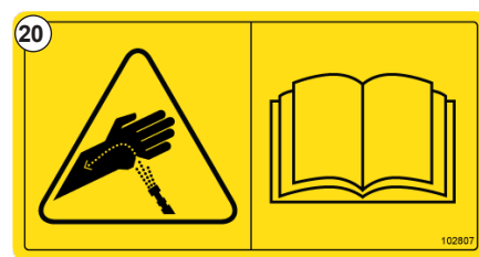
Fig. 23 - Do not pressure wash this area - #89333
