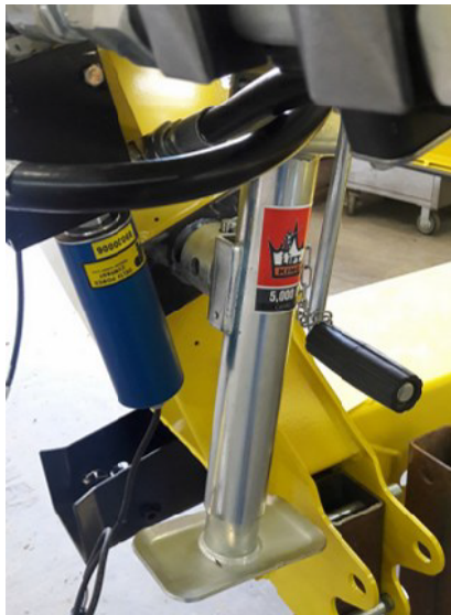
Fig. 35 - Jack stored on side of strut
