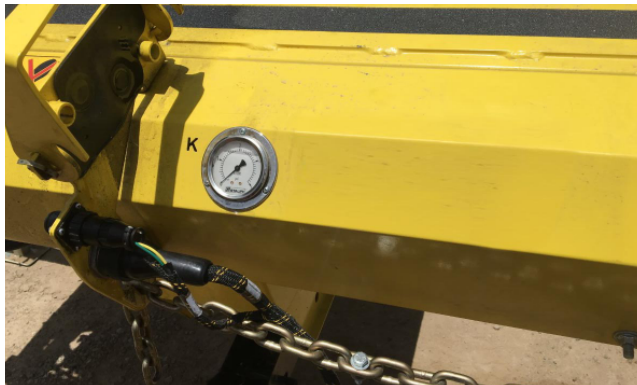
Fig. 46 - Hydraulic pressure gauges
