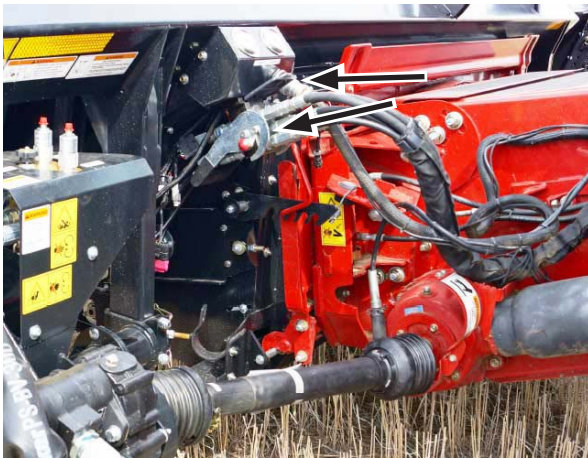
Fig. 31 - CONNECTING HYDRAULICS & ELECTRICAL
