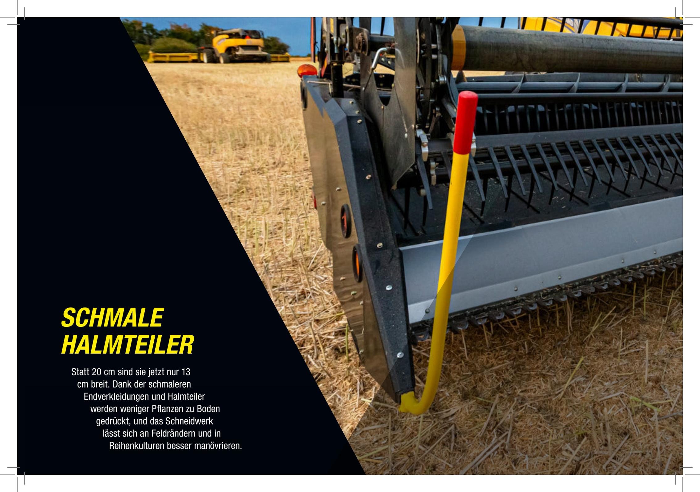
A close-up photograph of a combine harvester's straw divider mechanism. The divider is a dark grey metal structure with a prominent yellow and red safety handle. It is positioned over a field of harvested grain, with a yellow tractor visible in the background under a clear blue sky. The image is partially obscured by a black diagonal overlay on the left side, which contains text.
