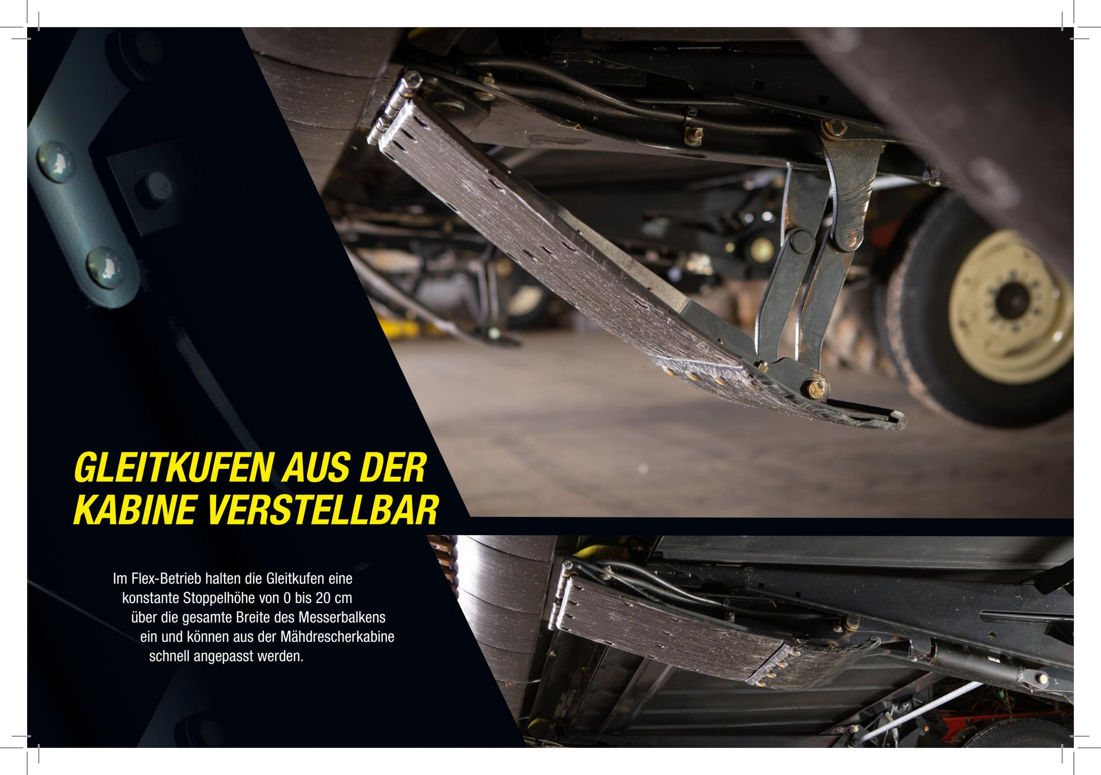
The image shows a detailed view of the sliding shoe mechanism on a combine harvester's cutter bar. The sliding shoe is a long, curved metal strip with a textured surface, mounted on a complex metal frame. It is designed to adjust the cutting height of the harvester. The background shows the internal components of the harvester, including a yellow wheel and various mechanical parts.
