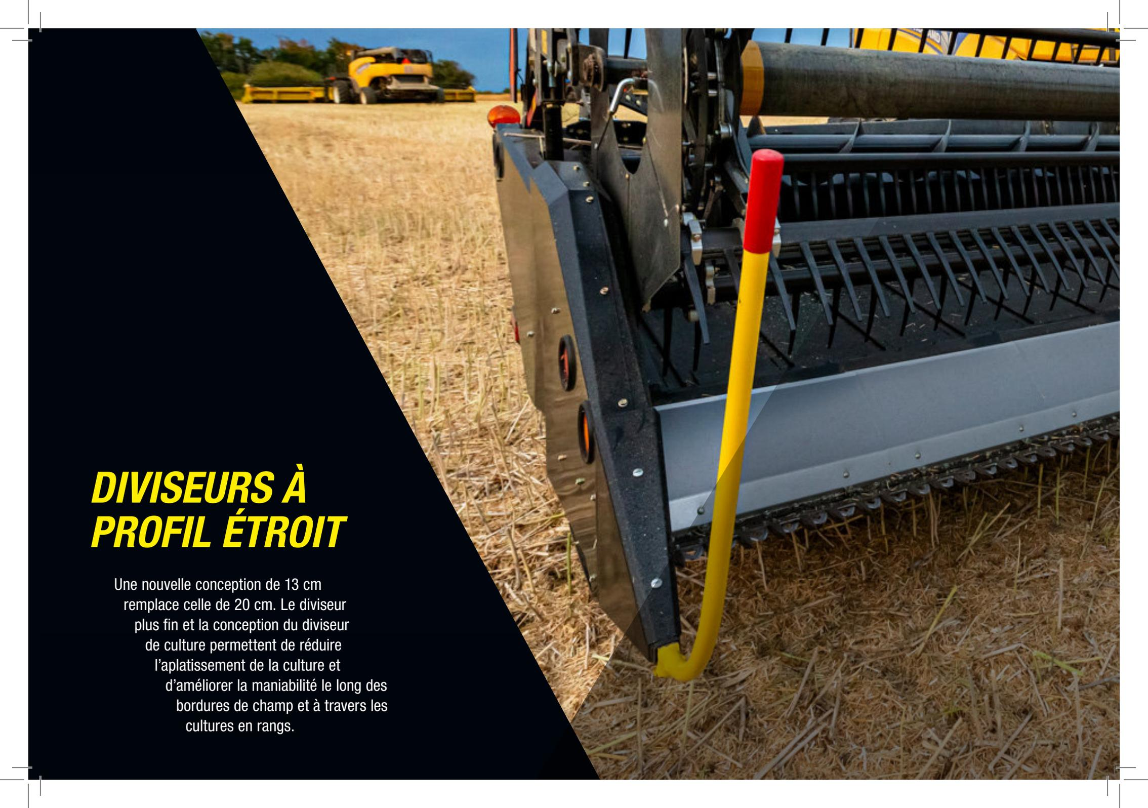
A close-up photograph of a harrow's narrow profile divider. The divider is a dark, metallic, L-shaped component with a red and yellow safety handle. It is positioned in a field of harvested crops, with a yellow tractor visible in the background. The divider is designed to be 13 cm wide, replacing a previous 20 cm design.
