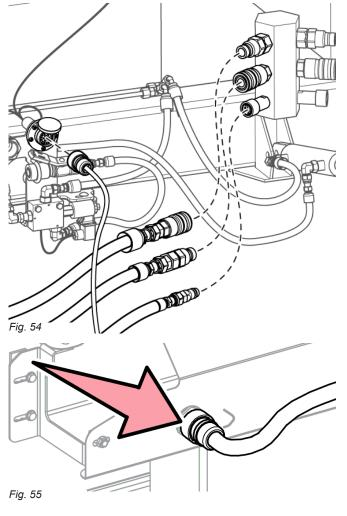
Locate the reel lift quick coupler on the storage bracket. Secure it to the quick coupler on the bracket that was installed on the front of the windrower as shown below.
