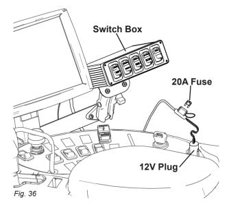
Secure the external harness to the connector on the outside of the cab as shown below. Route the harness under the cab between the fuel tanks. Secure the harness along its length using zip-ties.
