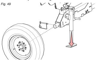
3. Remove the quick pin securing the hub and spindle, and remove the wheel assembly. Store the wheel assembly in an appropriate location, or if the gauge wheel option is present, install the wheel into one of the gauge wheel mounts and secure with the quick pin.
