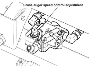
Fig. 141 - Cross auger flow/speed control
