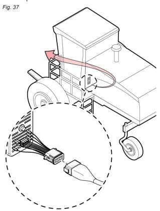
11. Secure the connectors on the end of the harness as shown below.
