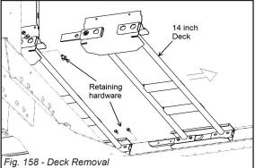
15. Re-install the formed plate with eyebolt into the channel of the main deck.
