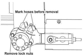
Fig. 104 - Driver Roller Removal
