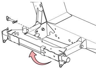
Fig. 60 - Axle in Field Position
