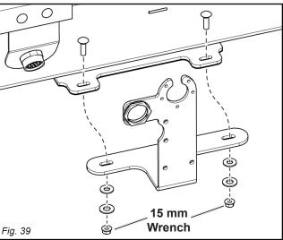
13. Secure the 21 pin plug from the external harness and dust cap to the bracket using #10-32 x 1" machine screws, #10-32 nuts and #10 star lock washers (5 ea.) as shown below. Add the provided O-ring (27449) under the dust cap.
