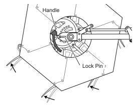
Fig. 89 Less Aggressive Finger Pitch (HB Reel)
