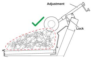
Fig. 137 - Adjust hold-down clearance to cutting section
