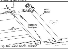
Before tightening the retaining hardware, make sure that the end of the formed plate is butted-up against the stop on the mount, and that the nut is against the face of the formed plate. **Do not**
