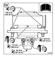
Fig. 22 Decal - Knife drive maintenance
