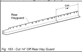
19. Using the retaining hardware, re-install the shortened rear hay guard at the end of the existing middle section of rear hay guard. Reinstall the chain mount on the rear side of the deck. Do not re-install any hose clamps.
