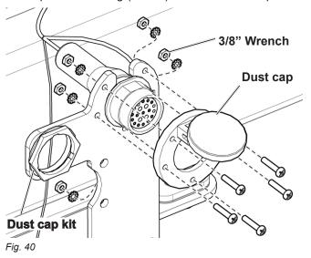
14. Plug in the other 21 pin plug from the external harness to the location shown below.
