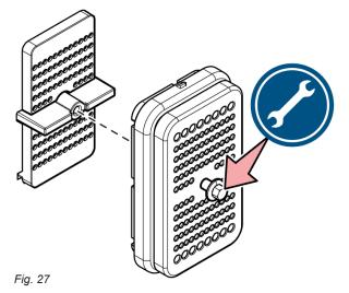
3. Remove the two wedge locks from the rear of the connector as shown below.
