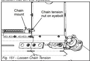
8. Remove the retaining hardware and first section of rear hay guard from the deck. The chain mount (with chain attached) on the rear side can hang down for now.
