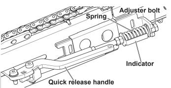
Fig. 98 - Deck Tensioning
