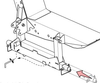
Fig. 59 - Axle Tube Retraction
