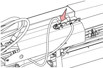
Fig. 56 - Reel lift quick coupler
