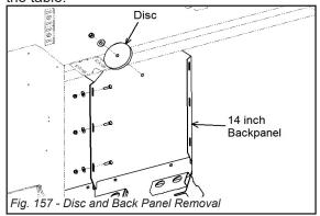
14. Remove the retaining hardware and 14 inch deck (with connectors) as a unit from the table.
