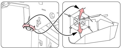
Fig. 85 - Reel Height Adjustment
