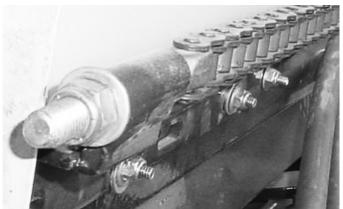
Fig. 144 - Roller Chain Tensioner
