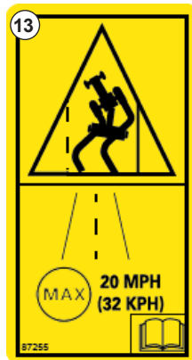
Fig. 15 - Crash warning, do not exceed 32km/h (20 mph) - #87255
