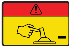
Fig. 136 - Warning! Dump air!
