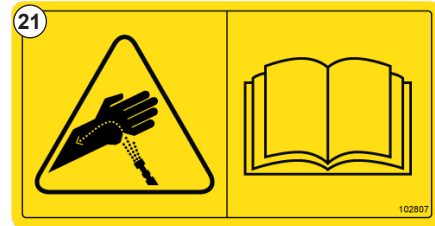
Fig. 23 - High pressure fluid warning - #102807
