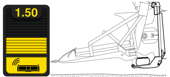
Fig. 135 - Sensor Bar Graph - Header pushed up
