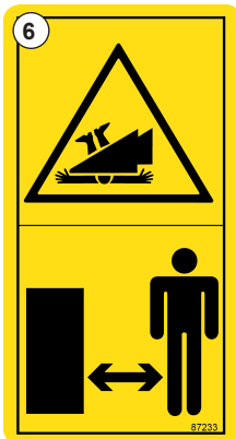
Fig. 8 - Crush warning keep safe distance - #87233
