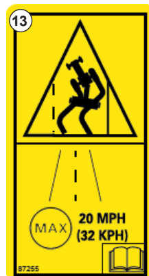
Fig. 15 - Crash warning, do not exceed 32km/h (20 mph) - #87255
