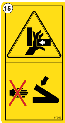
Fig. 17 - Pinch warning, keep away from moving parts - #87263
