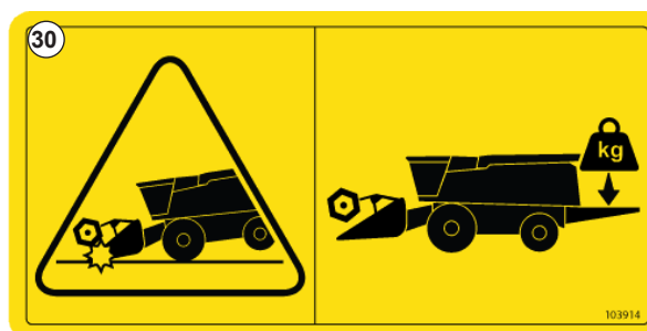
Fig. 32 - Tip warning, ensure combine is properly ballasted prior to operating - #103914
