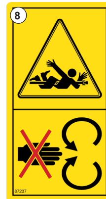
Fig. 10 - Rotating shaft warning do not touch - #87237
