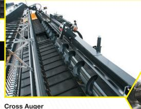
Hydraulic drive cross augers assist in material flow from the drapers to the feed auger. The auger is adjustable to match varying crop conditions and increases combine capacity in bulky crops like peas and mustard. Augers are 'size' specific.
