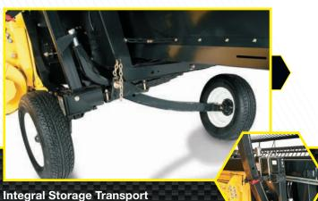
The self-contained integral transport including hitch, jack and axle is conveniently stored on the header table.
