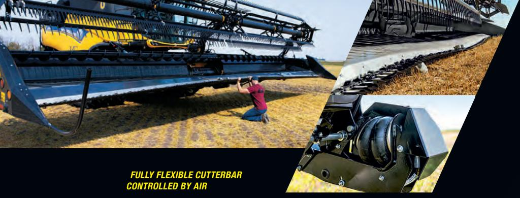
The independently-suspended cutterbar is light, fast-reacting, and infinitely adjustable.
