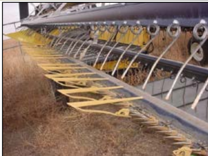
Crop Lifters Installed - Illustration A - Page 130
