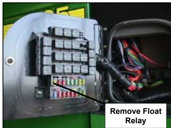
Illustration D - Page 50: Electrical Panel - Float Relay
