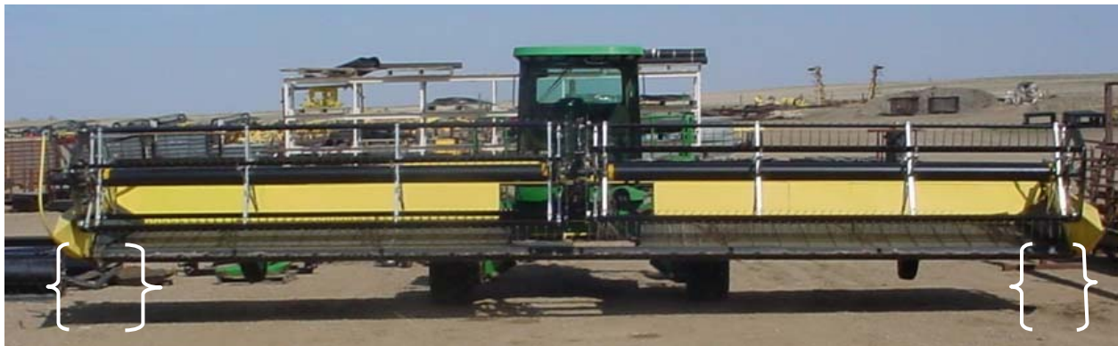
Measure the end clearance, adjust reel until it is centered. Figure 40.6
