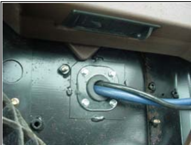
Illustration 3-34: Wiring Installation Complete
