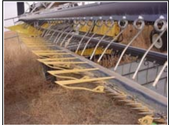
Illustration 11-17: Crop Lifters Installed
