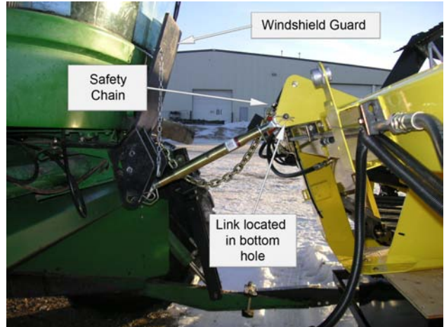
Illustration 57: Manual Lift Link
