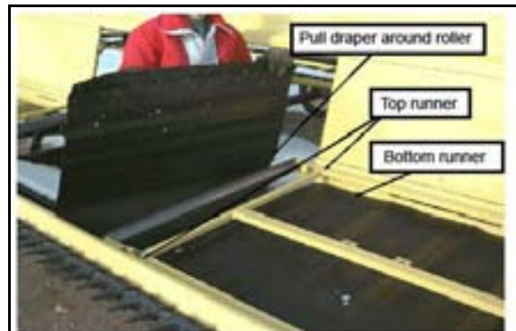
Illustration 6-2: Feeding Draper onto Bottom Runner
