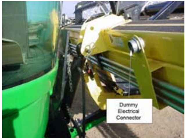
Illustration 4-8: Transport Electrical Connector
