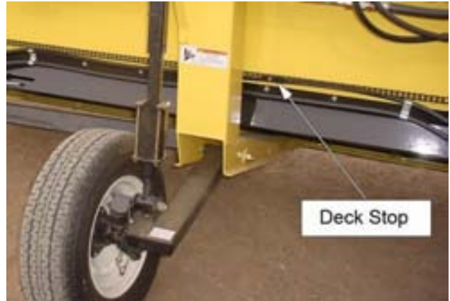
Illustration 11-8: Deck Shift Stops
