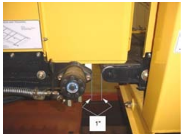
Illustration 11-9: Setting Deck Gap
