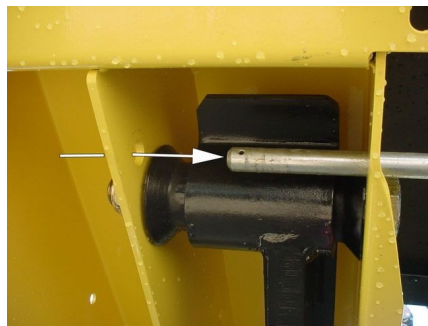
Illustration 82: Removing the Hitch Pins
