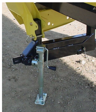
Illustration 81: Axle Jack in Position
