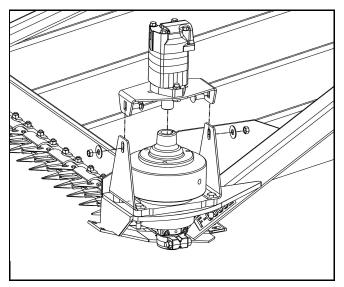
5. Remove the hydraulic motor from the knife plate as shown to the right.
