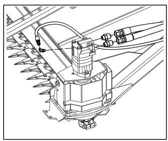
3. Remove the knife drive shield and the set screw as shown to the right.
