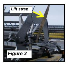
**Step 2:** Remove reel lock retaining pin.
