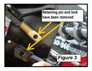
**Step 3:** Install replacement reel arm lock bar and replace pin, both right and left side.
