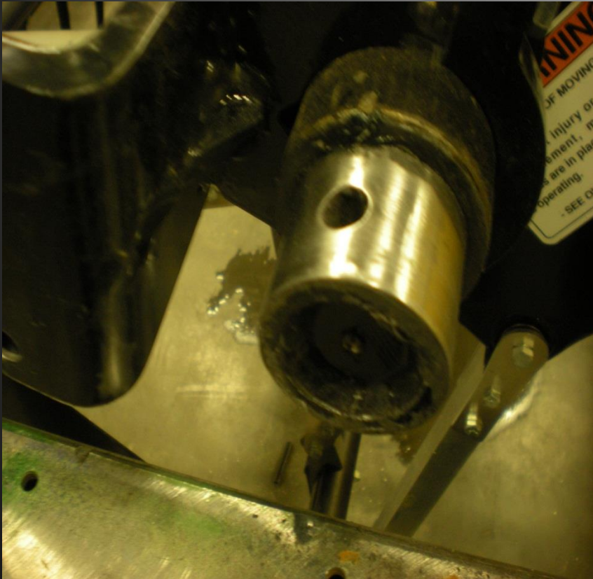
CLEAN SHAFT SURFACE FOR NEW COUPLER INSTALLATION.
