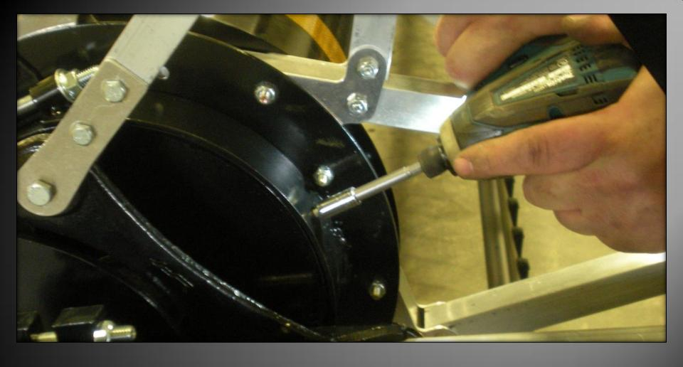
ADD THE SELF TAPPING SCREWS (6 PER SIDE) IN THE HOLES PROVIDED. REPEAT ON OPPOSITE END OF THE CENTER TUBE.
