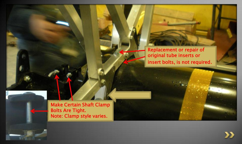
REMOVE BOTTOM ROW OF BOLTS NEXT TO THE CENTER TUBE FROM THE REEL ARMS. REUSE NUTS!
