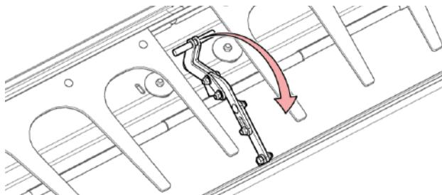
Рис. 252 - Open Rock Trap at Center Draper
