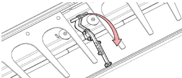
Рис. 235 - Open Rock Trap at Center Draper
