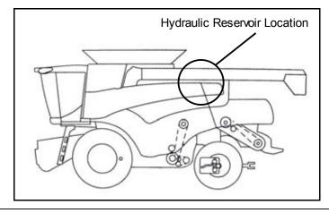
2. Remove the hose from the return port on the combine hydraulic reservoir.
