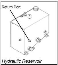
3. Install the tee fitting into the return port on the hydraulic reservoir.
