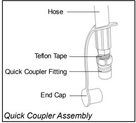
9. The hose plugs into the quick coupler located at the upper left corner of the sub frame.
