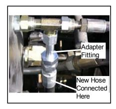
7. Run the hose along the existing hydraulic lines. Continue to the front of the combine, securing with zip-ties along the way. Do not route the hose along any location where it may become damaged through contact with moving parts.
