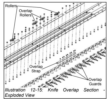
The overlap sections (on the overlap strap), and the right hand knife back should be tight to each other when the counter sunk bolts are tight.
