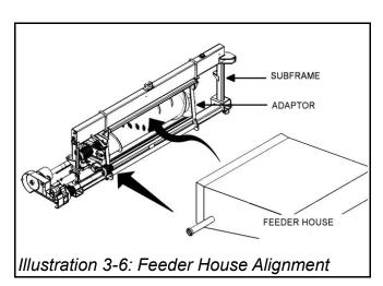
the header either up or down to improve alignment. Adjust feeder house height as needed.
