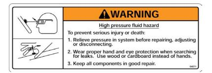
You can reduce this hazard by relieving the pressure before disconnecting hydraulic lines, and by tightening all connections before applying pressure.
