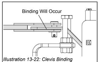
Ensure that the link arm is adequately spaced from the bearing assembly on the sensor mount, so that it moves freely and does not rub against the sensor mount.
