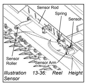
8. With the cutter bar at its lowest position, the sensor arm should point slightly down and be located on the front side of the sensor assembly.
