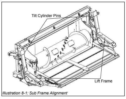
3. Move forward slowly, paying special attention to the alignments mentioned on the previous page. Ensure that the tilt cylinder pins will barely clear the bottoms of the mounting plate notches. If the sub-frame is too much lower than this, you may encounter interference between the guide plate sides and the mounting plate notches.
