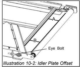
Once extended, you should make sure that everything is parallel. The easiest way to do this, is to measure the distance between the roller and the closest cross brace on the draper deck. Make sure measurement "A" is the same distance as measurement "B". If it still does not line up, you may adjust the eye bolt again.
