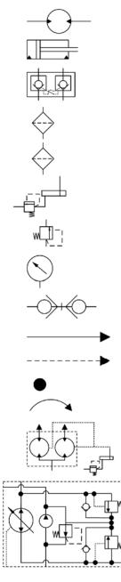
Hydraulic motor – fixed displacement, reversible.
