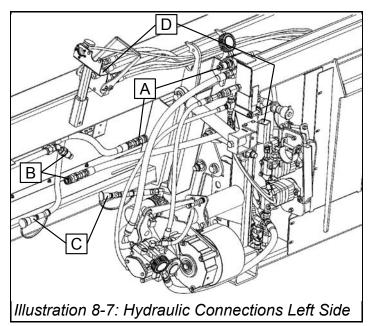
11. Locate the header tilt cylinder valve on the left side of the frame, and connect the pressure line for the header tilt cylinders here. When connected, turn the valve to "on" position by moving the lever to the right.
