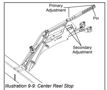
When servicing the reel, it is necessary to have the reel locked into the servicing (highest) position, with the lock pins securely in place.
