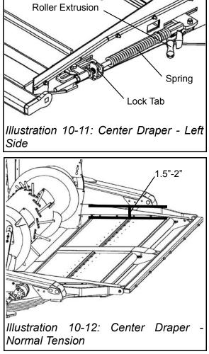
Normal adjustment of the center draper would provide 1.5" - 2.0" (3.8 cm - 5.0 cm) of slack in the center of the draper (when measuring vertically from the top of the draper runner on the inside of the deck, to the top of the draper).
