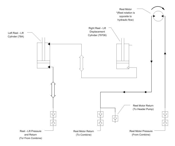
Split – Reel Lift Circuit with Double Reel Drive (42 and 45 ft Headers)
