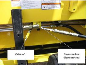
Illustration 7-6: Header Tilt Valve - Closed
