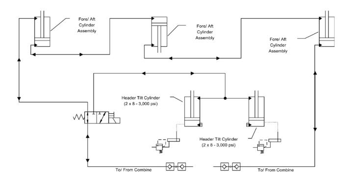
Hydraulic Fore & Aft with Hydraulic Header Tilt Assembly (Solid Reel)
