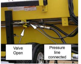
Illustration 7-5: Header Tilt Valve - Open
