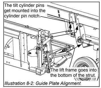
4. When the tilt cylinder pins are directly below the mounting plate notches and the lift arms are fully inserted into the frame struts, slowly raise the sub-frame until the tilt cylinder pins are fully seated in the mounting plate notches.
