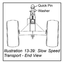
5. Using the jack, lower the header hitch onto the mounting pin on the top of the slow speed transport. Replace the quick pin and washer to secure.
