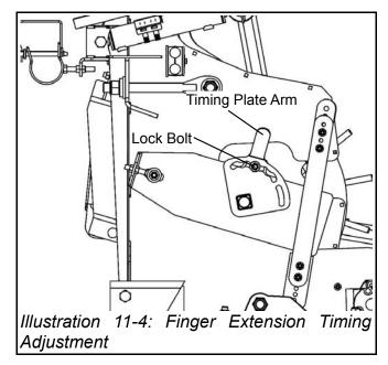
Normal adjustment of the fingers is to have them fully extended at the two or three o'clock position (viewing the auger from the right-hand end of the tube.).
