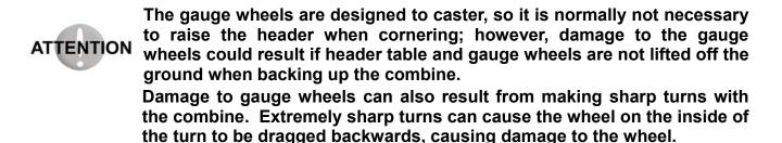
The gauge wheels must be adjusted relative to the height at which the header will be operated in the field. Normal adjustment would allow the weight of the header to compress the spring shaft of the gauge wheel assembly approximately 1.5" (38 mm) to 2.0" (50 mm).
