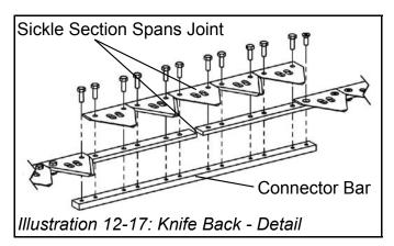
The joint in the two knives must be centered under a full sickle section, with the connector bar centered underneath the joint.
