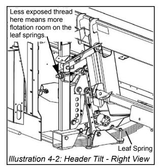
To lower the cutter bar relative to the sub-frame, extend both adjuster bolts. This adjustment will provide more clearance between the sub-frame and the ground; and will also provide more clearance between the feeder deck and the ground. This setting will bring the cutter bar closer to the ground. \*(See Examples 4-3 through 4-6)
