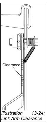
If the sensor arm is too close or rubs on the sensor mount, it may be necessary to install one or more spacers (washers) behind the rod locking collar. Do this by first loosening the bolt on the inside of the sensor mount, then removing the rod locking collar. Next add spacer(s) into the pocket behind the locking collar, and re-assemble. Re-check the alignment and spacing between the sensor rod and sensor arm.
