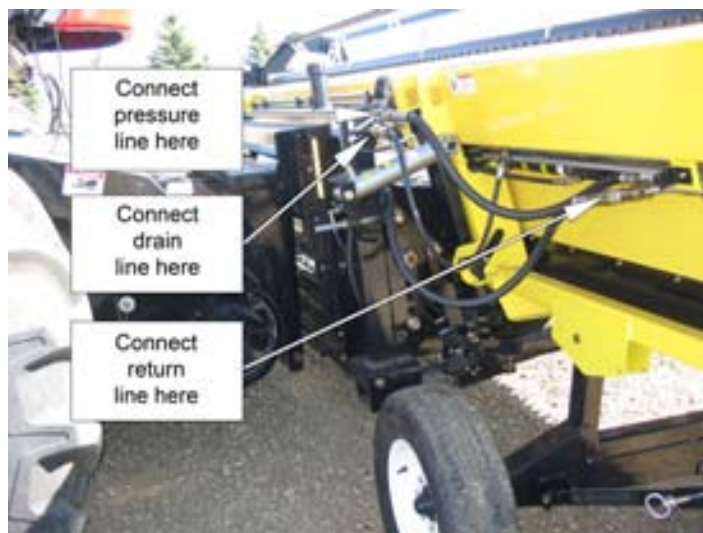
Illustration 8-6: Connecting Right Side Hydraulics
