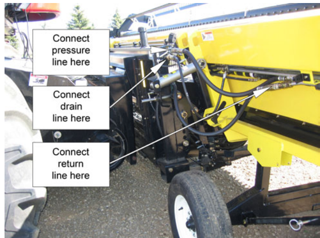
Illustration 98: Connecting Right-hand Side Hydraulics
