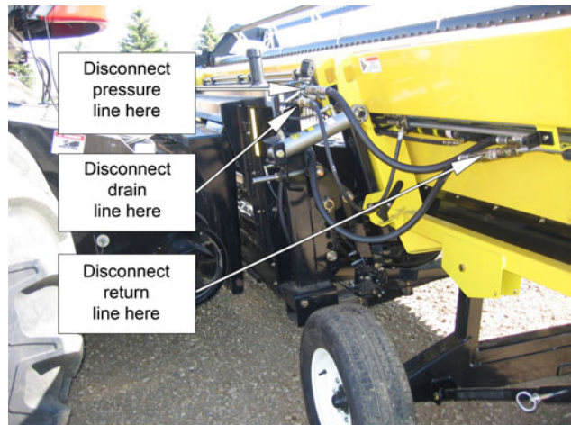
Illustration 88: Hydraulic Disconnects - Right Side
