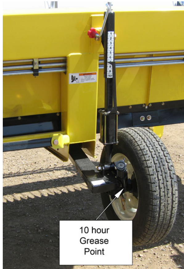
Illustration 103: Gauge Wheel Lubrication Point
