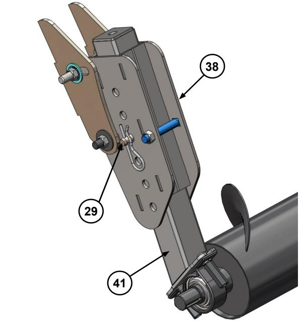
Install **Right Hand Cross Auger Assembly** by sliding **U-Joint (22)**, on left end, onto the **Right Hand Shaft of the Center Cross Auger Assembly**. Then slide the **Slide Tube (41)**, on the right end, into the **Adjustment Bracket (38)**. Place **Lock Pin (29)** into the hole shown on the previous page. Leave all fasteners loose for final adjustments.
