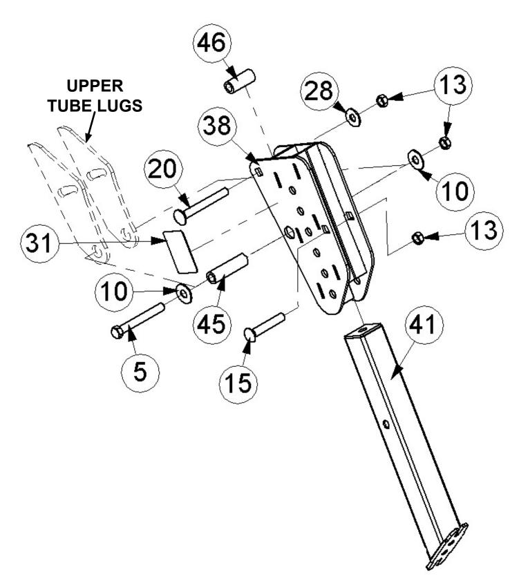
Gather parts, numbered below, and assemble on the **Right Hand Cross Auger Weldment (42)** preparing it to be attached to the **Right Hand Adjustment Bracket** (38) and **Center Cross Auger**. Use a good **Anti-Sieze Compound** on all connections involving the auger shafts.
