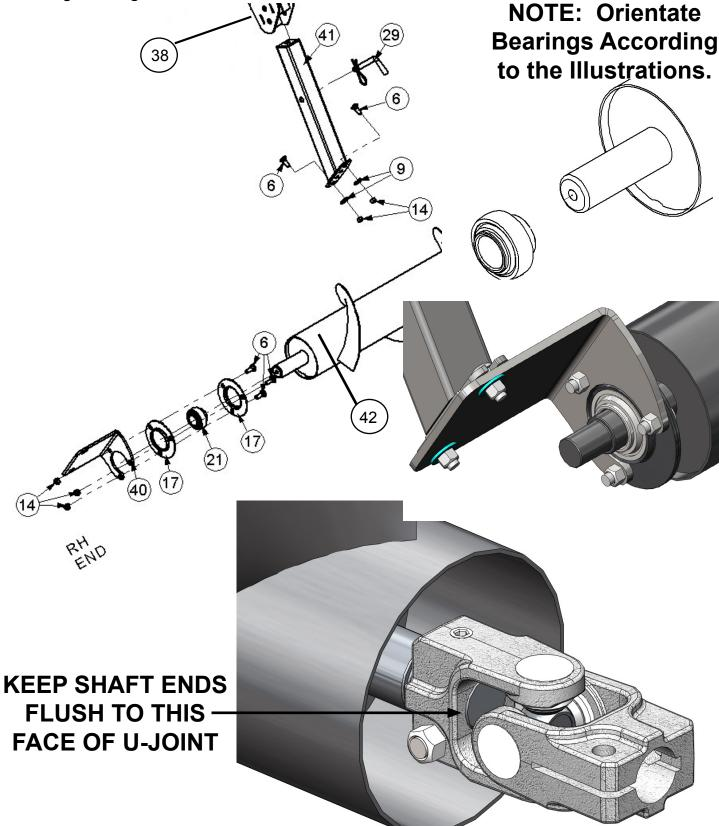
Gather parts, numbered in the illustration, and assemble on the Center Cross Auger (35) preparing it to be attached to the Right Hand Cross Auger Assembly, Left Hand Cross Auger Assembly, and the **Inner Adjustment Brackets** (38). Do not forget the Anti-Sieze.
