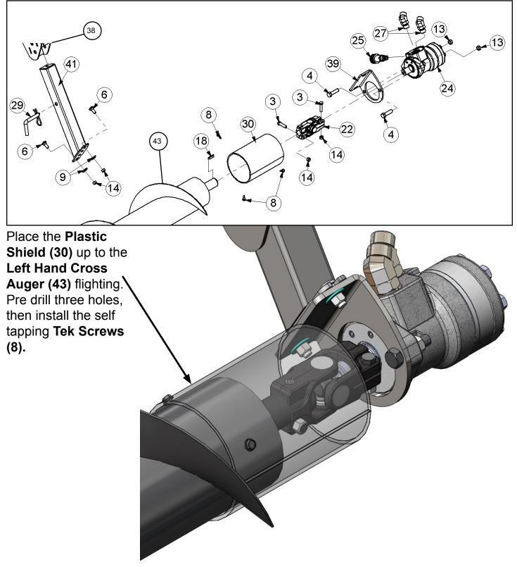
Install Center Cross Auger Assembly by sliding the Left and Right Slide Tubes (41) into the Adjustment Brackets (38). Place Lock Pin (29) on each side into the hole shown below. Leave all fasteners loose for final adjustments.
