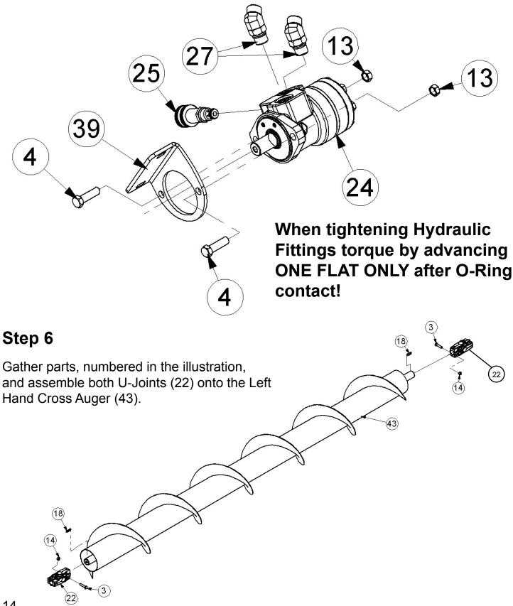
Gather parts, numbered below, and assemble on the Left hand Cross Auger Weldment (43) preparing it to be attached to the Left Hand Adjustment Bracket (38)
