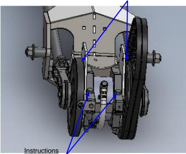
Remove the  $2 - \frac{1}{2} \ge 5 \frac{1}{2}$  gr. 5 unc. bolts. Replace bolts with  $2 - \frac{1}{2} \ge 5 \frac{1}{2}$  gr. 8 unc. Torque bolts to 120 ft.lb. Note: If gr. 8 bolts are not available torque existing bolt to 120 ft.lb.
