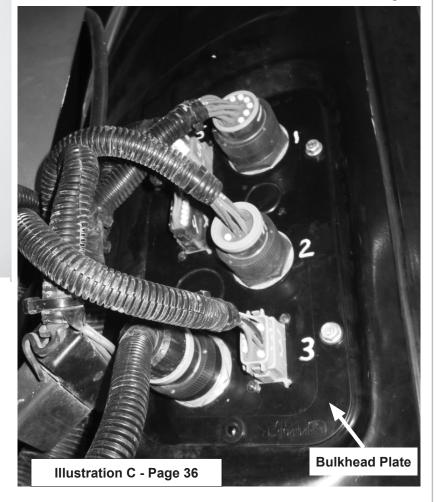
To route the Switch Box Cable in the cab, first remove the Bulkhead Plate (Illustration C) from the Outer Right Rear of the cab.
