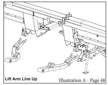
7. Slowly raise the lift arms and move forward until the arm extensions are firmly set into the mounting boots (see illustration B). Ensure the end of the extension arm has fully engaged the mounting boot and the locking arm has dropped into the proper position. Do not lift the table any higher at this point.
