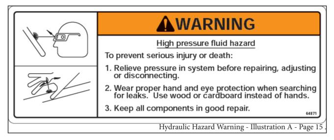
You can reduce this hazard by relieving the system pressure before disconnecting hydraulic lines. Once finished, tighten all connections to specifications before re-applying pressure.
