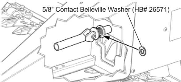
Fig. 250 - Add washer to tighten loose handle
