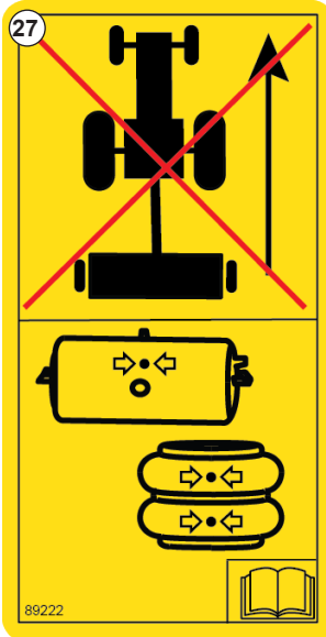
Fig. 31 - Pressurise air system to RIGID mode before transporting - 89222
