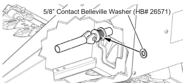
Fig. 246 - Add washer to tighten loose handle
