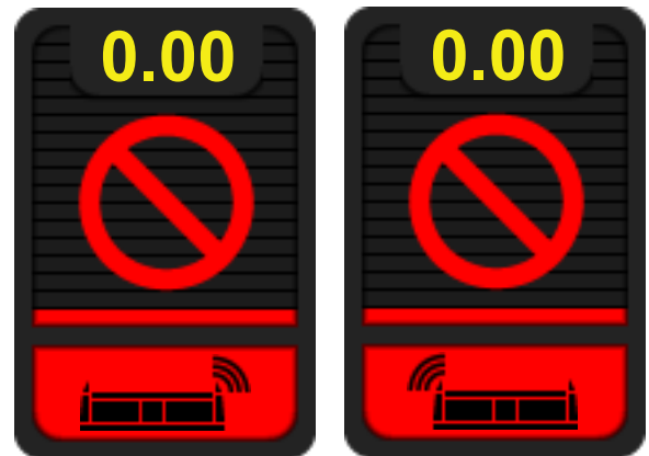
Fig. 146 - Warning! Header height sensor not detected!
