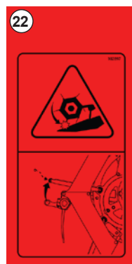
Fig. 25 - Secure reel tines before operating - #102897
