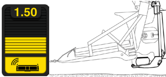
Fig. 143 - Sensor Bar Graph - Header pushed up
