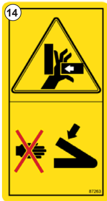
Fig. 17 - Pinch warning, keep away from moving parts - #87263
