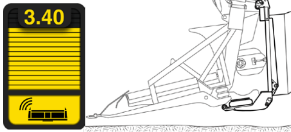
Fig. 142 - Sensor Bar Graph - Header full range available
