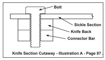
The knife sections must be installed on the top side of the knife back (the side stamped "TOP") so that the protruding inserts of the connector bar will fit snugly into the tapered section holes. As the section bolts are tightened, the inserts in the connector bar are drawn into the knife back forcing them to clamp down on the bolt. The bolts should be tightened to 120 - 150 in-lbs, (13.5 - 17 Nm).
