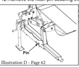
14. Install the transport axle jack to support the weight at the rear of the table.
