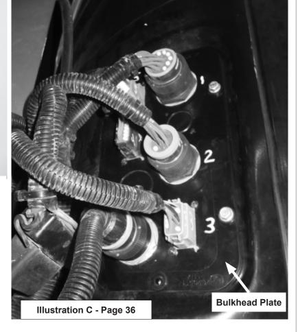
To route the Switch Box Cable in the cab, first remove the Bulkhead Plate (Illustration C) from the Outer Right Rear of the cab.
