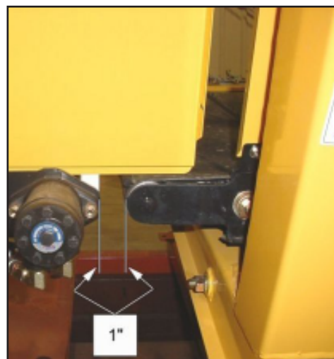
Setting Deck Gap- Illustration B - Page 127 .
