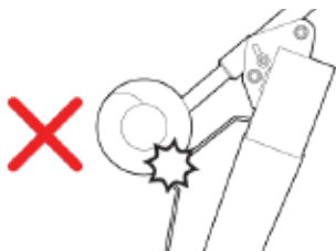
Fig. 68 - Cross auger impacting back panel
