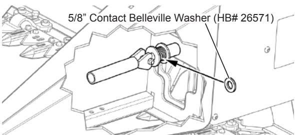
Fig. 197 - Add washer to tighten loose handle
