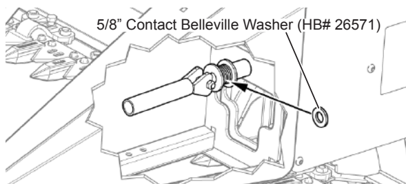
Fig. 202 - Add washer to tighten loose handle
