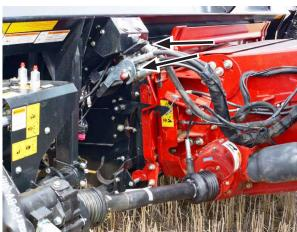
Fig. 31 - CONNECTING HYDRAULICS & ELECTRICAL
