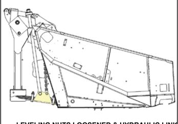
LEVELING NUTS LOOSENED & HYDRAULIC LINK SHORTENED - Illustration B - Page 35Honey Bee Manufacturing Ltd. 4000 Series Header
