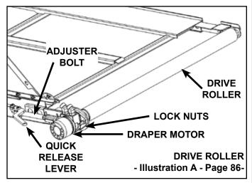
5. Check bearing in end of roller, and remove any build up of material on roller.
