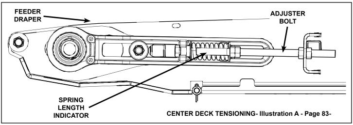
Draper tension can be easily modified by adjusting both Spring Tensioned Pushrods on either side of the **Feeder Draper** independently. Loosen or tighten the Draper by turning each sides **Adjuster Bolt**.
