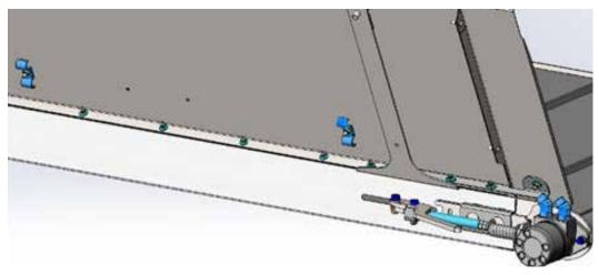
6. Manually shift both the left hand and right hand deck inward approximately 7.0" (18 cm). Then shift the middle deck inward until there is approximately a 1.5" (3.8 cm) gap between the left hand and middle deck drapers. This insures there is enough clearance for the draper slats during operation.
