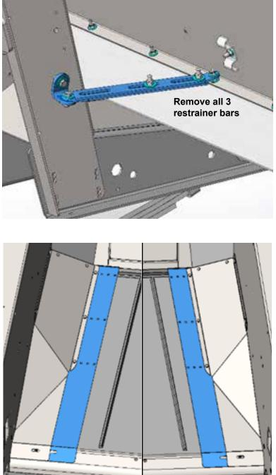
4. Shift both the RH and LH deflector extensions to outmost position.
