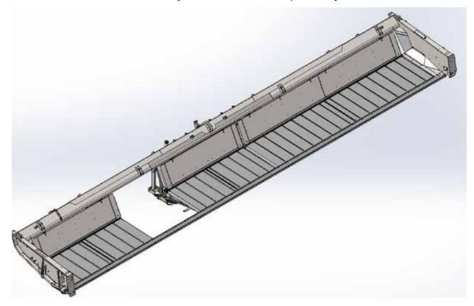
The header will outfitted from the factory with three decks instead of two so that the middle deck can be manually shifted either right or left. From the factory the header will be setup to function as a typical combine header (i.e. the middle deck will be shifted to the right hand side). To convert to the manual swath mode please follow the steps below:
