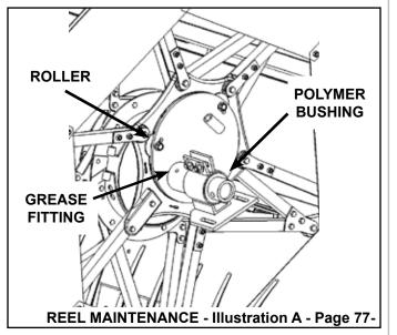
The control ring assemblies each have three rollers mounted in adjusting slots. To compensate for wear to the control ring, the rollers may be adjusted outward in the slots so that all three rollers are lightly in contact with the control ring.
