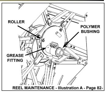
The control ring assemblies each have three rollers mounted in adjusting slots. To compensate for wear to the control ring, the rollers may be adjusted outward in the slots so that all three rollers are lightly in contact with the control ring.
