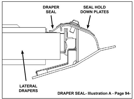
The Seal Hold Down Plates should push down the seal onto the Lateral Drapers with enough pressure to lightly touch the Drapers.
