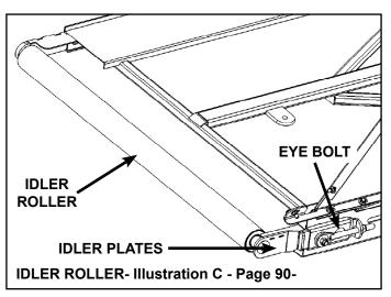
7. Re-assemble in reverse order. See *"Idler Roller Tracking Adjustment" on page 86*, adjust tension and tracking as necessary.
