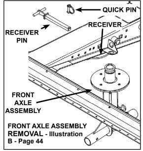
10. Mount the Front Axle Assembly in the Front Axle Assembly Storage Bracket, on the Header Frame as shown. Secure in place with Lock Pins.
