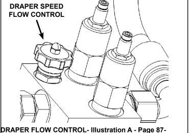
The speed of the Lateral Deck Drapers and the Center Deck Draper is controlled by an adjustable flow control in the Main Manifold Block. Adjusting the **Draper Speed Flow Control** will affect all Decks. When using the Header as a Swather the Draper speed should be set to form a good Windrow, to remove the cut crop from the Cutter Bar and to deliver it smoothly to the opening.
