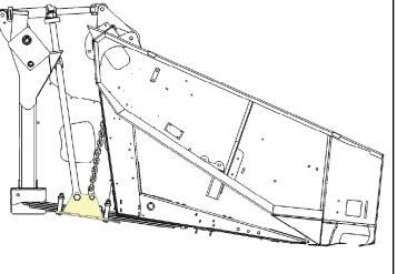
LEVELING NUTS LOOSENED & HYDRAULIC LINK EXTENEDED - Illustration A - Page 39-
