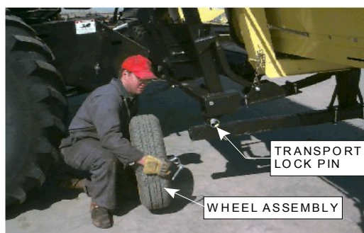
Illustration 44: Rear Tire Removed
