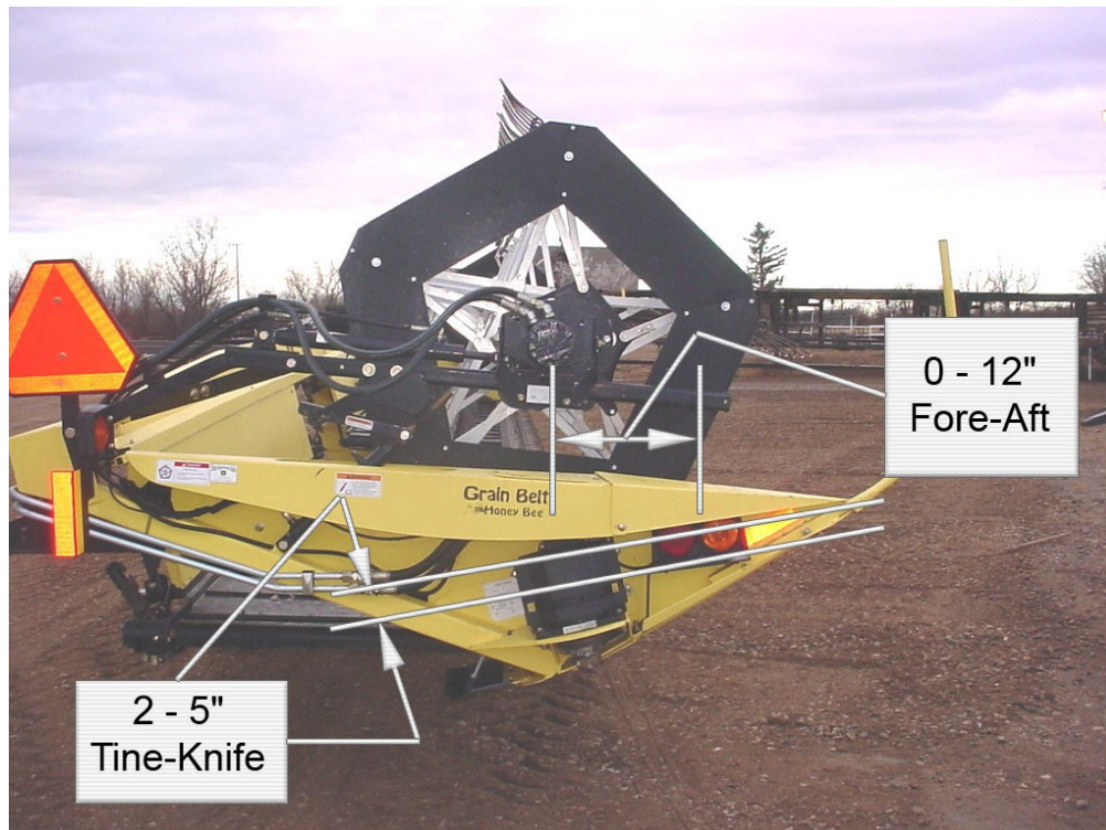
Illustration 102: Reel to Knife Measurements
