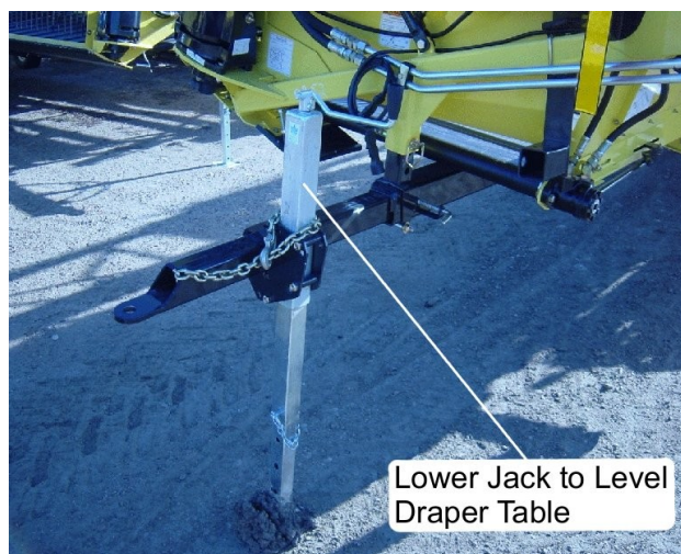
Illustration 147: Leveling the Table
