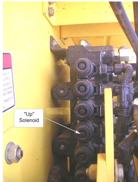
Illustration 2: Hydraulic Solenoids - Front View
